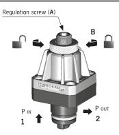
The regulator Series TC regulates and maintains the air pressure to the desired value, which can obviously not be higher than the line pressure. In order to regulate you need to turn the regulation screw (A), rotating it clockwise or anti-clockwise, in any case the right regulation of the pressure has to be set upwards and then block the rotation. The air flow has to follow the direction from "1" to "2". Use the nut (B) to block the regulation and avoid accidental setting changes.
