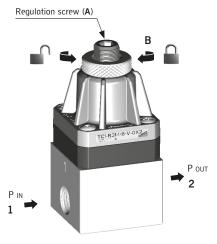
When installing the regulator cartridge on its sub-base or in a seat made for a specific customer application, insert the O-ring (C) and then fix the regulator cartridge using screws (**D**), both supplied.
