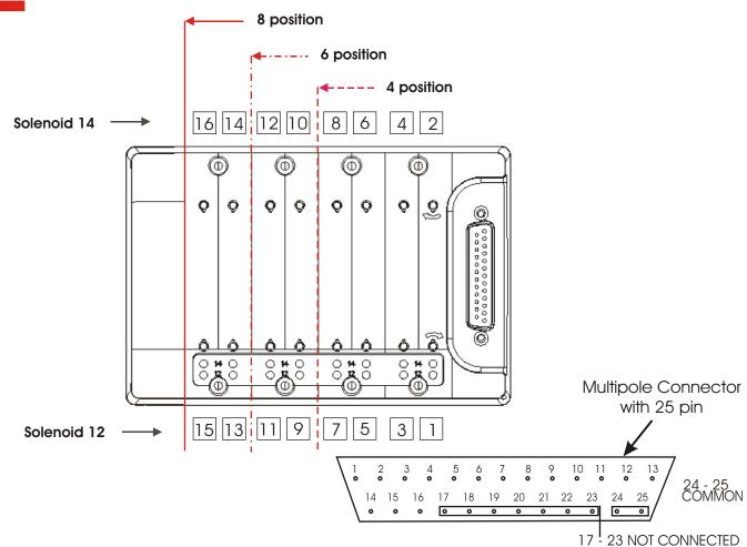
Corrispondece between: the position of the solenoid and the valve outlet of the valve for the different valve function
